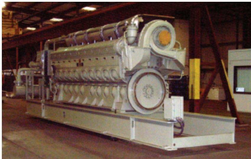
An EMD 20-cylinder 645E3B stationary generator set engine ready for conversion to the Haynes UltraFire ERS Emission Solution Kit.
