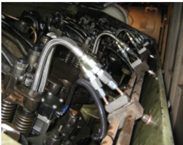
Haynes UltraFire ERS electronic injector with EnviroTip technology applied to an EMD 16-645E3B locomotive engine.
