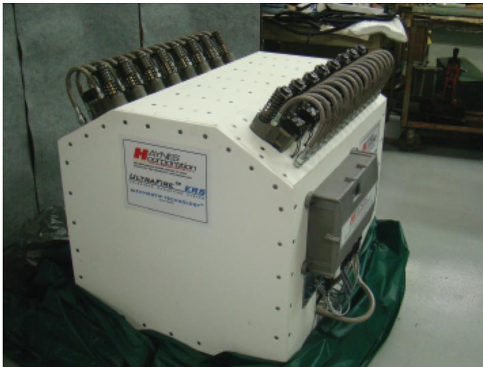
Haynes Corp. has introduced the UltraFire ERS Kit, a retrofit emissions reduction system targeting stationary, rail and marine engine applications. Shown here is a display system at the company's Naples, Fla., shop.
